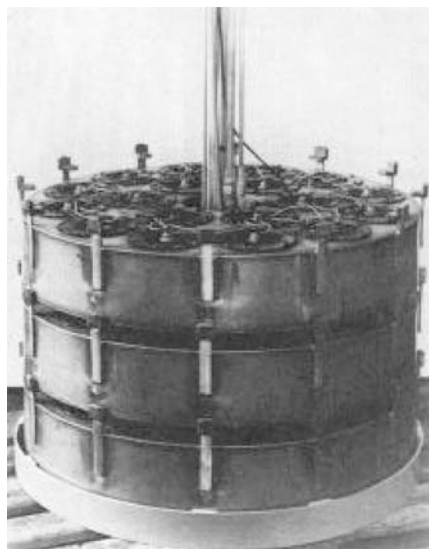
Fig. 2 Three coils of a 10-cell, 60-W methanol–air battery with cylindrical air diffusion electrodes for a flashing sea buoy [4]
